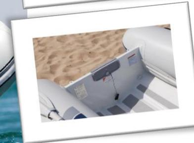
Hull : 2.5mm thick powder coated marine grade aluminium
